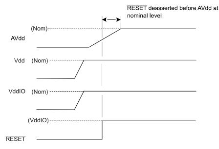
The RESET pin can be used to reset the device whenever necessary. The RESET pin must be asserted low for at least 90 ns to cause a reset. After releasing the RESET pin the device typically takes 93 ms before it is ready to start communications. It is recommended to connect the RESET pin to a host controller to allow it to initiate a full hardware reset without requiring a power-down.
