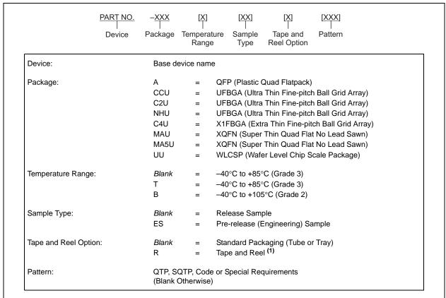
Note 1: Tape and Reel identifier only appears in the catalog part number description. This identifier is used for ordering purposes and is not printed on the device package. See "Orderable Part Numbers" below or check with your Microchip Sales Office for package availability with the Tape and Reel option.
