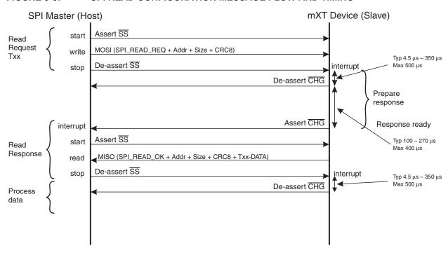
Normally a limit of 64 bytes is allowed for data reads. If the host tries to read more than 64 bytes, the slave returns SPI\_READ\_FAIL (see Section 9.4.3 "SPI\_READ\_FAIL"). A mechanism is provided, however, that supports the DMA transfer of a large block of data that exceeds this limit. This is achieved by the provision of multiple instances of the Data Container T117 object within the device that allow up to 1290 bytes of data to be read in a contiguous manner.
