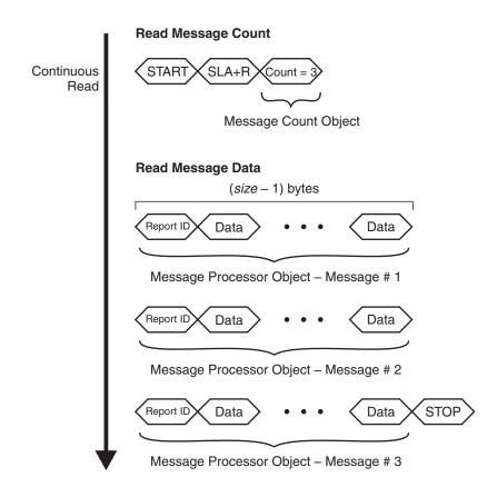
FIGURE 8-5: CONTINUOUS MESSAGE READ EXAMPLE – I<sup>2</sup>C CHECKSUM MODE
