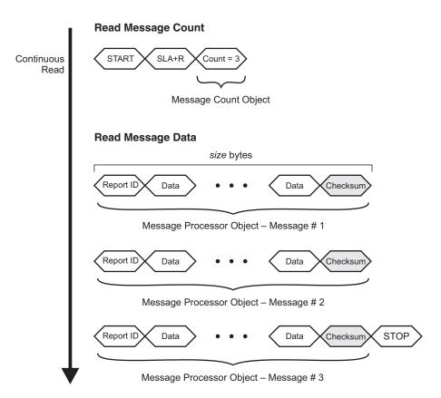
There are no checksums added on any other  $I^2C$  reads. An 8-bit CRC can be added, however, to all  $I^2C$  writes, as described in Section 8.3 " $I^2C$  Writes in Checksum Mode".
